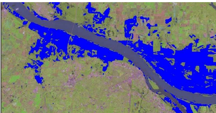
Sample flood map generated with rapid flood mapping technique that identifies newly inundated areas, which will assist emergency management agencies to quickly locate areas that need assistance.
