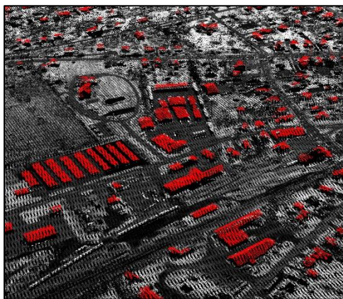
VermontView developed algorithms to map buildings from 3D lidar data in Middlebury, VT to support solar potential estimates.
