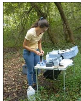
Lauren Roberts is using the mobile test kits to test for pH, conductivity, iron, copper, aluminum and hardness. She will presenting her results at a Spring 2022 Conference
