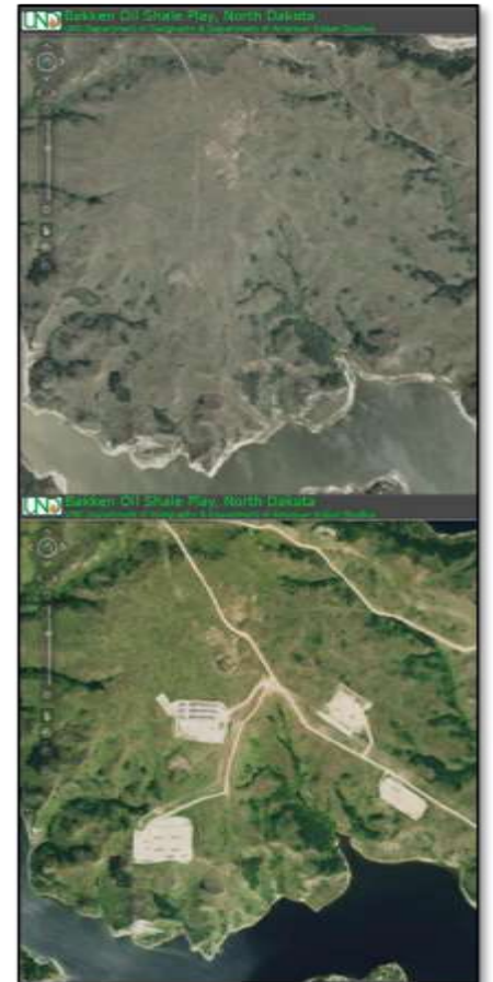
An example of land-cover change associated with the Bakken Oil Boom. The top image was acquired in 2003 and the bottom in 2014, showing the development of several oil well pads. Source: USDA NAIP
