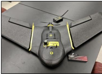
Picture of a senseFly eBee UAS used to collect imagery in this study. This is a light-weight, fixed wing platform capable of carrying a variety of sensors including both visible and multi-spectral cameras.
