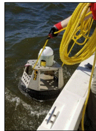
Monitoring water quality at depth using a custom-built sensor platform (PODs). After several weeks in the Mississippi Sound, the PODs are retrieved, analyzed, and compared to remotely sensed data.
