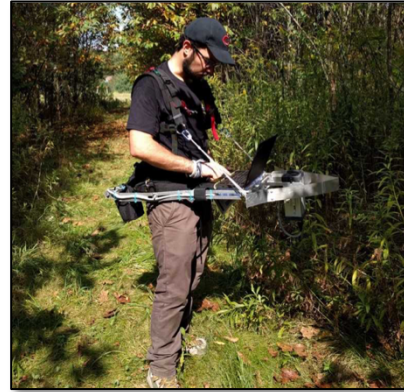
Portable Canopy Lidar (PCL) system being used to measure 2-D forest canopy structure. The PCL system is mobile and efficient for measuring canopy structure.
