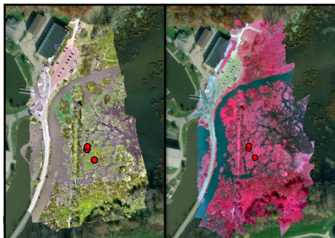
RGB and multi-spectral imagery, from a drone, of a wetland on Lake Erie to help identify types of vegetation for classification.
