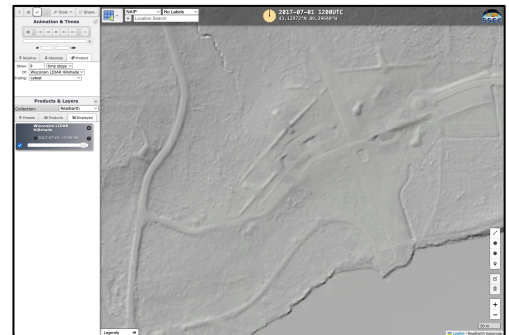
Shaded relief imagery derived from LiDAR displayed in RealEarth, showing earthworks in Wisconsin made by the Effigy Mounds Culture during the Late Woodland Period (1400-750 B.P.).
