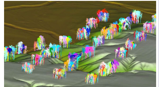
A Digital Terrain Model of a portion of Martell Forest populated by the individual trees extracted from terrestrial laser scans.
