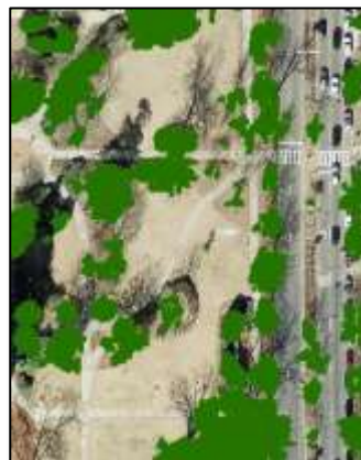
Shown above is an example of an urban tree canopy (left) dataset generated using both LiDAR and GeOBIA methods. Also shown is a rendering of a typical urban tree (right) using ground-based LiDAR laser scanning technology. These data are used in conjunction with airborne data for urban tree canopy identification and mapping.
