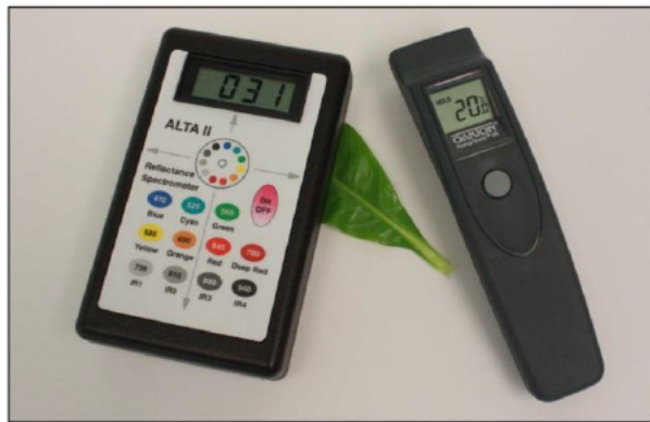
Left: The reflectance spectrometer and infrared radiometer included in the science kits to replicate the measurements made by the Landsat 8 spacecraft. Right: examples of leaf spectra made by a student during one of HawaiiView workshops
