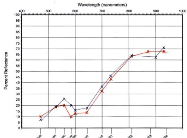
Left: The reflectance spectrometer and infrared radiometer included in the science kits to replicate the measurements made by the Landsat 8 spacecraft. Right: examples of leaf spectra made by a student during one of HawaiiView workshops
